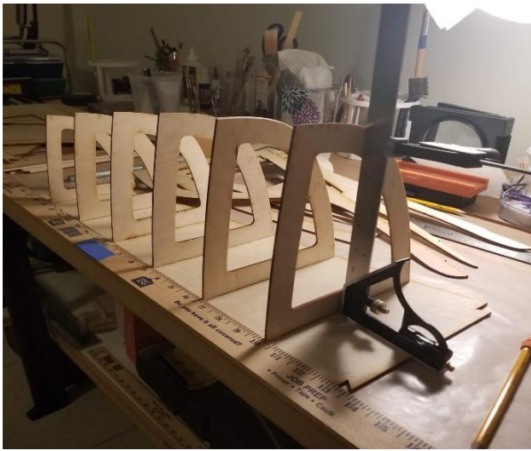
Sectional build of bulkheads on strong back
