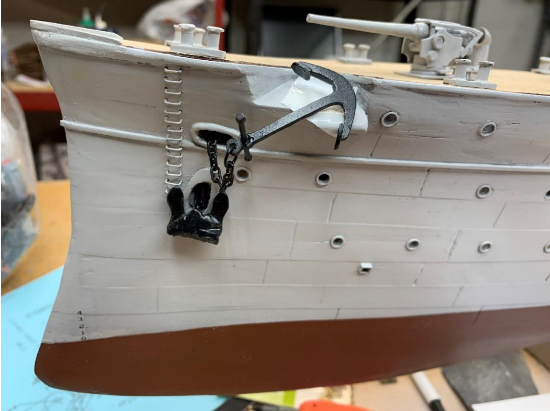
A good view of the over/under plating scheme
