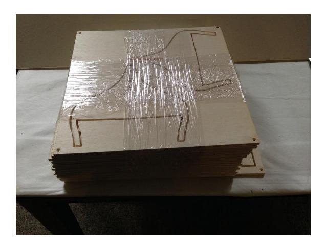
All 29 bulkheads, false keel and associated parts ready for bench work.
