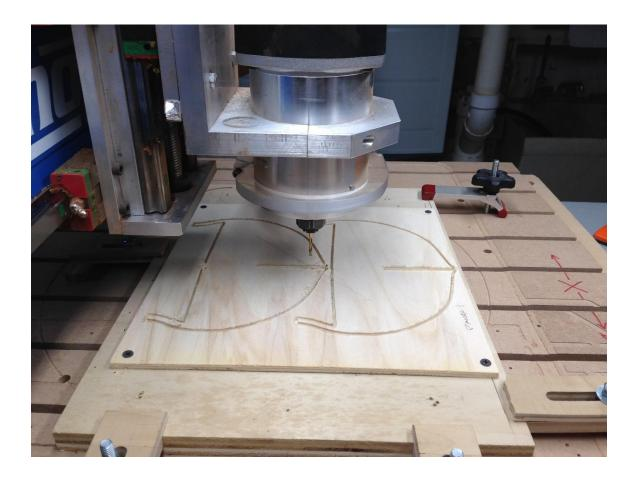
Two of the bulkheads on the Shop Sabre being machined out of <sup>1</sup>/<sub>4</sub> inch model plywood.
