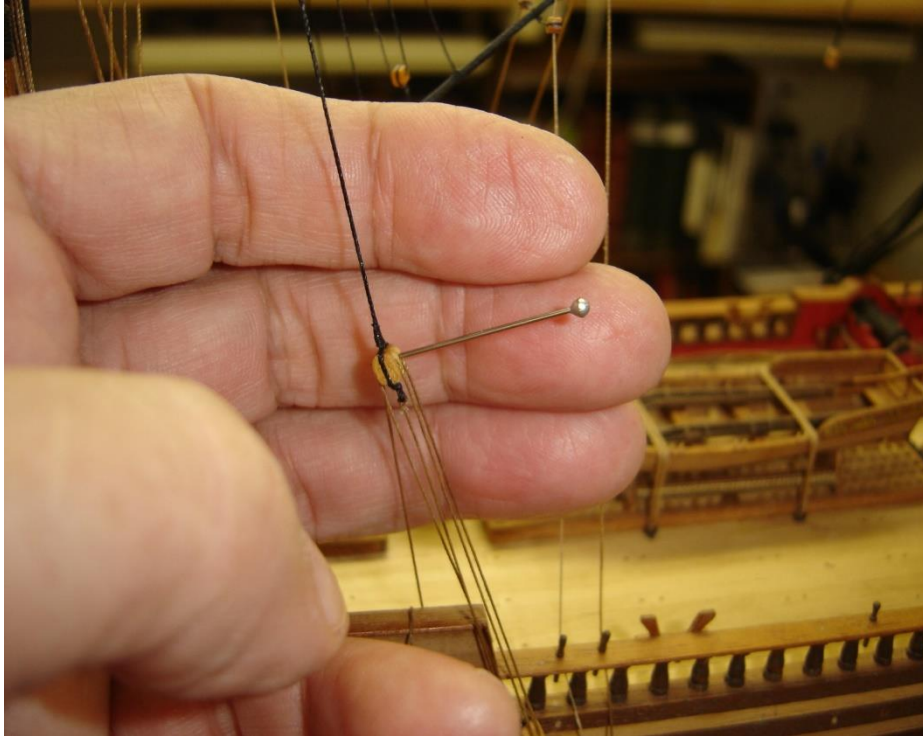
Temporary tensioning of rigging using straight pins
