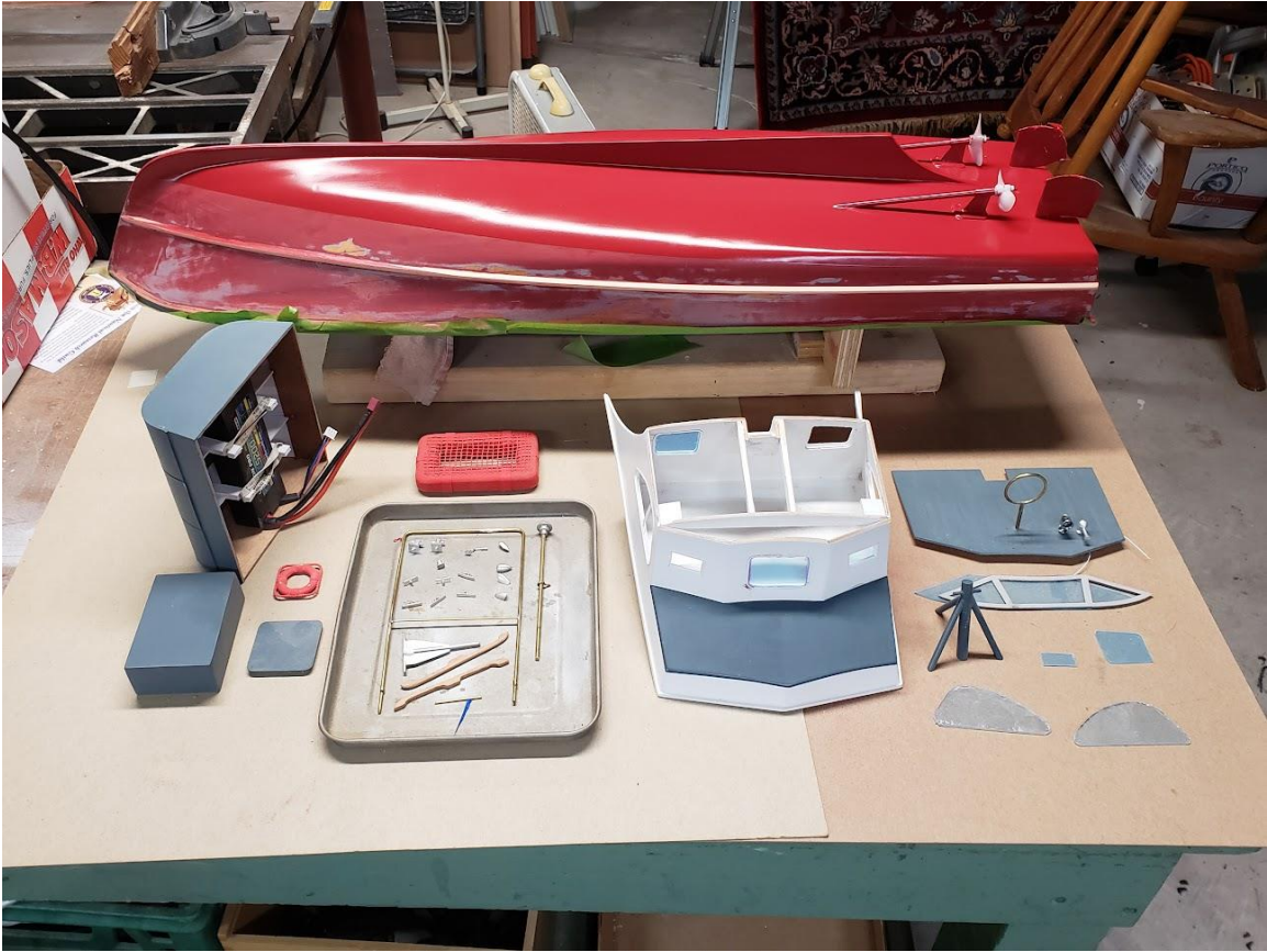
Some of the hull rework including the addition of the 2 nd prop, deck compartment that holds the battery, upended deck house and detail components.
